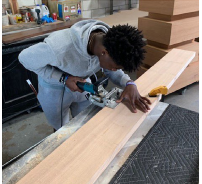
Sam Scaife is routing the edges of this board in preparation of joining several boards together.
